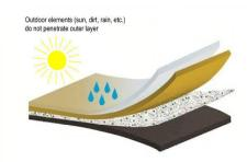
Figure 1. Advanced corrosion control covers protect against many agents.
