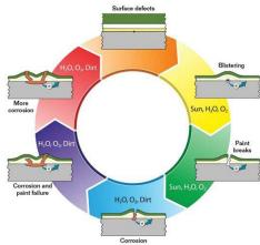
Figure 2. Paint failure and corrosion cycle.
